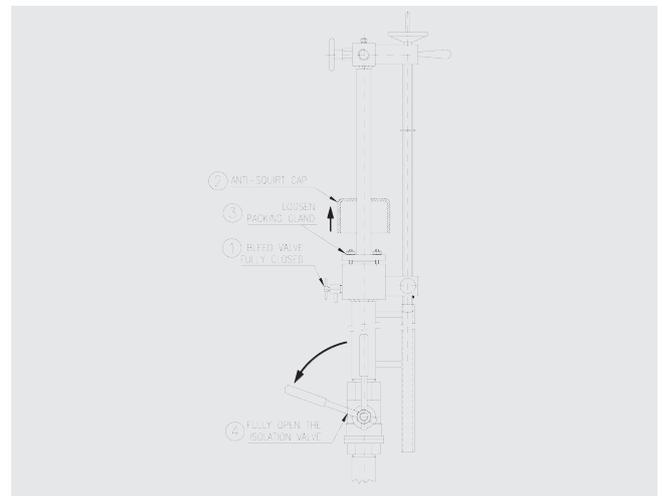
**Step 5:** Screw the anti-squirt cap on its original position and check that the isolation valve is fully open.
