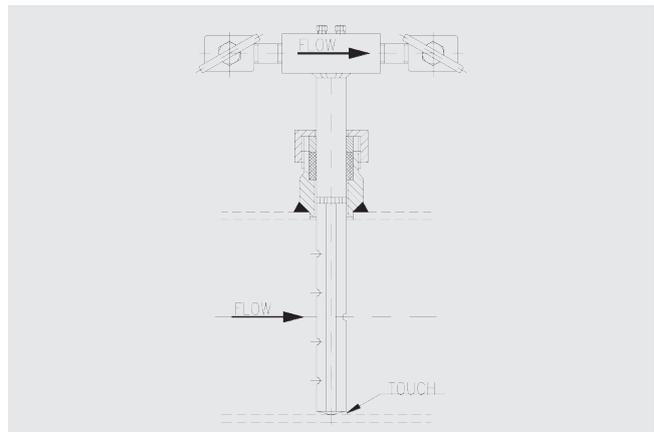
**Step 7:** Check the FloTec is installed correctly and aligned.
