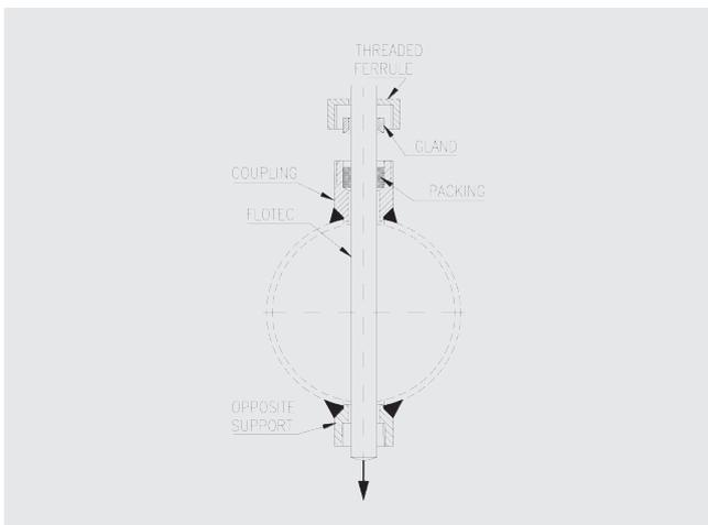
**Step 7:** Insert the FloTec with the threaded ferrule and the gland through the threaded fitting into the pipe and through the opposite support. Apply appropriate sealant and tighten the opposite support hex plug. Turn the FloTec until the flow arrow is positioned correctly and the sensor bar tip reaches the bottom of the hex plug.
