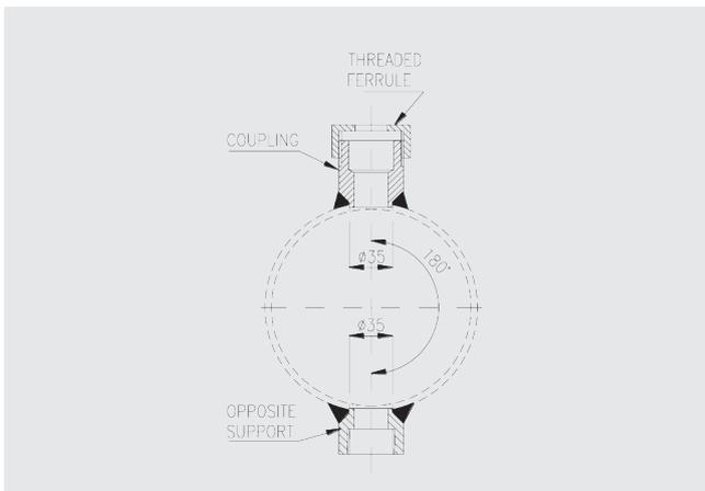
**Step 5:** Repeat steps from 1 to 3 to install the opposite support fitting.
