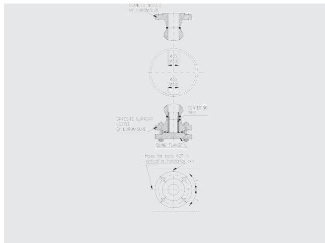
**Step 5:** Position the gasket onto the FloTec flange and carefully insert it through the flanged fitting (stand-off) until the two flanges mate squarely, ensuring the tip of FloTec enters the opposite support cup. Turn the upper flange until the flow arrow is positioned correctly. Fit the flange securing bolts and tighten equally and evenly, observing correct procedures
