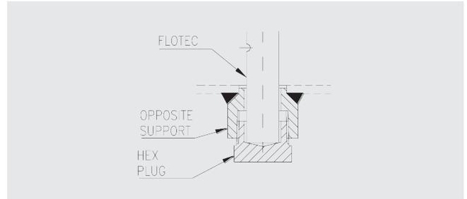
**Step 8:** Screw the compression fitting into the threaded fitting by tightening to 340 Nm torque. Holding the head of the FloTec with a wrench to maintain correct orientation, use a long wrench to tighten the compression fitting until approximately one thread is left exposed under the nut, ensuring the flowmeter does not turn.
