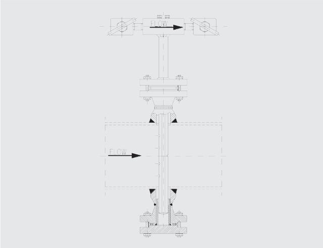
**Step 6:** Check the FloTec is installed correctly and aligned.
