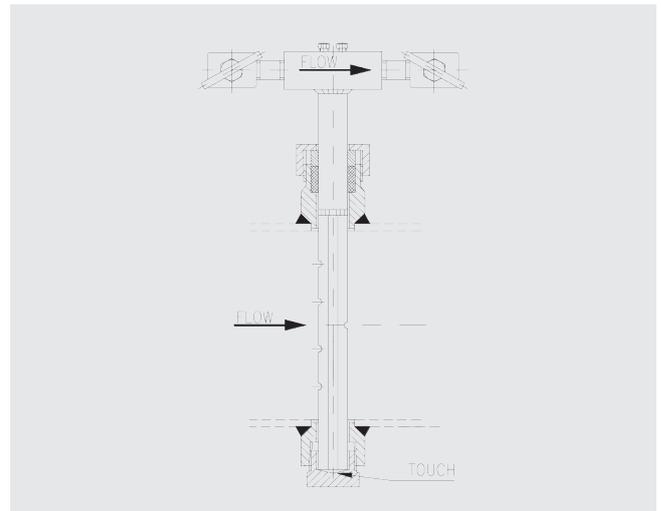
**Step 9:** Check the FloTec is installed correctly and aligned.
