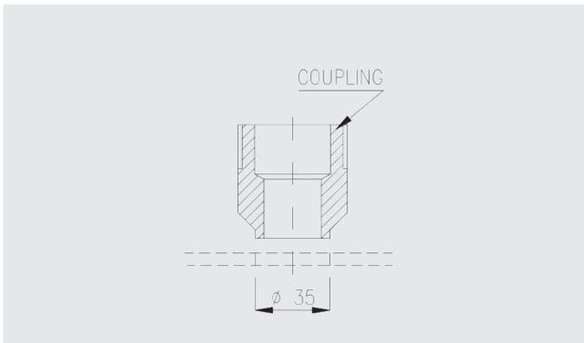
**Step 2:** Align the threaded fitting concentrically over the hole and tack-weld in place. Using a suitably sized and threaded length of pipe, check the threaded fitting is concentric and aligned correctly.
