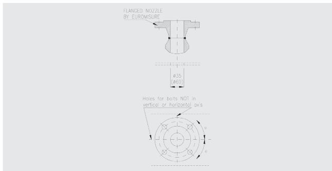
**Step 3:** Complete welding. Apply a full penetration root run completely around the base of the flanged pipe fitting (stand-off) at the clearly defined weld preparation line.
