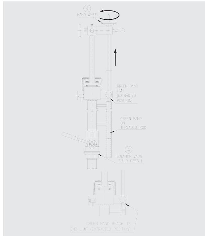
**Step 5:** Once Step 4 is completed, fully close the isolation valve (usually 1.1/2" ball valve type).
