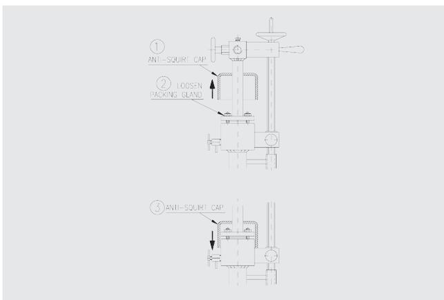
**Step 4:** Turn the handwheel till the green band painted on the threaded rod reaches its end limit (extracted position).
