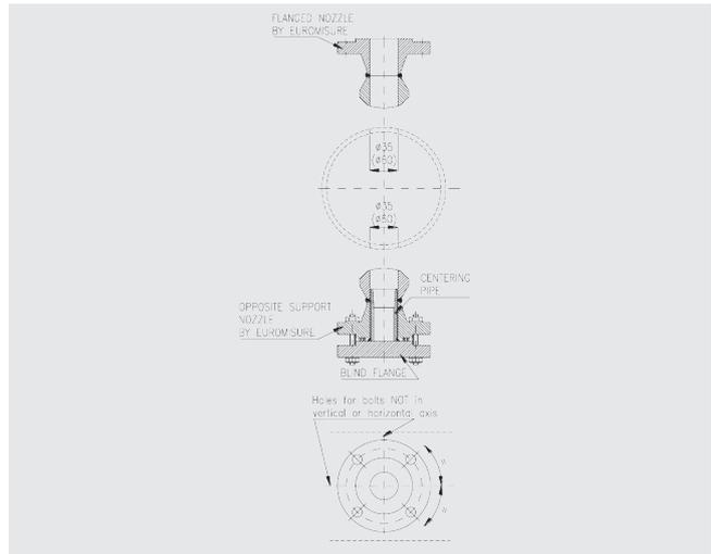
**Step 4:** Insert the FloTec through the nozzle into the pipe and check that the tip protrudes through the hole in the opposite pipe wall when the two flanges mate squarely. Position the end-support cup over the tip of the flowmeter, ensuring the tip is concentric with the hole, and tack-weld the end-support cup in place. Remove the FloTec and complete the support cup weld.
