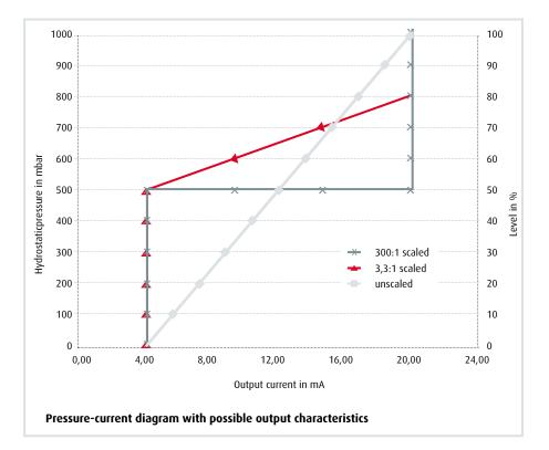
range of the instrument, the scaled range, at about one third, is relatively small. It would almost be minimal if one had taken a turndown factor of 300:1. Translated into the tank example, with a possible pressure profile of 1000 mbar, at 300:1 the operator would thus be wanting to measure just about 3.3 mbar. In other words, a maximum measuring height of ten metres would shrink to a total of 33 mm.
